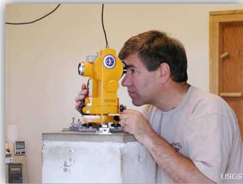
This surveyor is using a theodolite.
